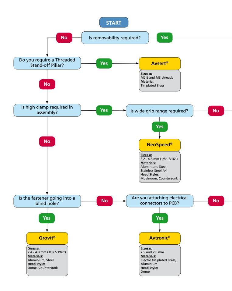
This selection guide is designed to illustrate which fasteners may be the most suitable for your application. This guide does not include the full range of POP Avdel products; our Applications Engineers are available to advise as to the best solution for your specific application needs.
