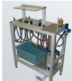
8-head station with adjustable rivet modules for the assembly of transformer and starter to base plate of a fluorescent lamp
