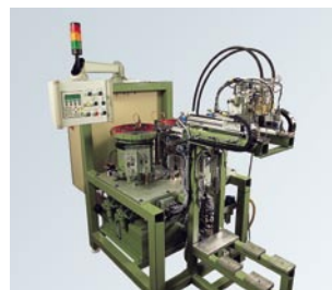
MIRS system with two riveting heads to assemble vacuum pump
