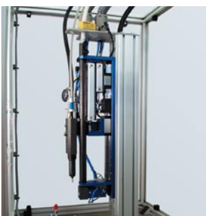
Avimat® automated assembly system The compact, lightweight placing head can be mounted separately and work in any position - for maximum production flexibility
