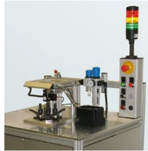
Adjustable 4-head MAS assembles two types of seat belt retractors; on two positions modules are adjustable against stopper
